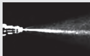
Injector spray pattern before P.i. treatment.
